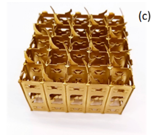
Grid spacer after application of surface nitriding
