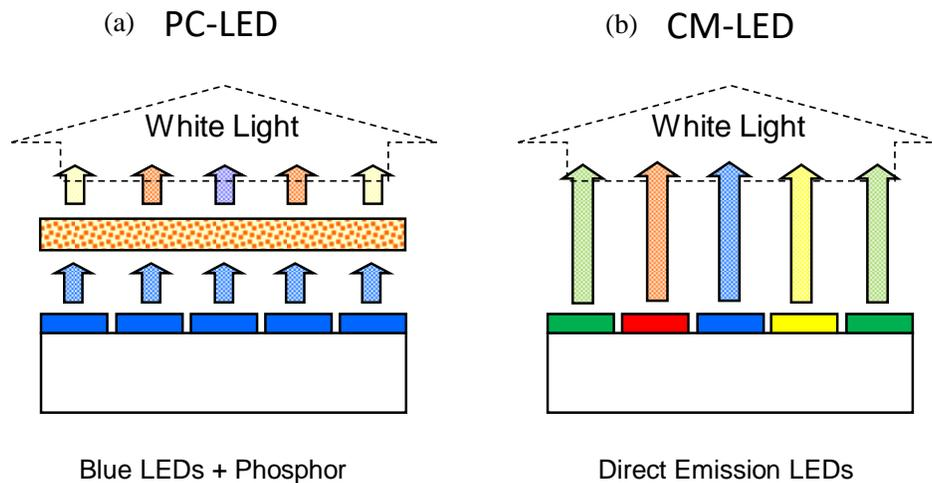
Figure 5-1. Schematic of Two Main White LED Architectures
