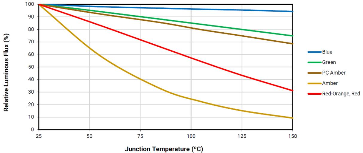
Figure 5-7. LED Efficiency as Function of Junction Temperature [16]
