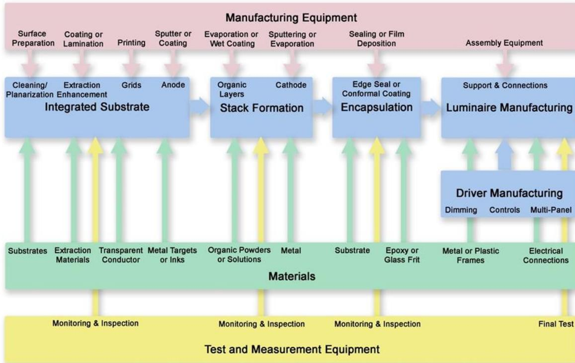
Figure 7-4. OLED-Based SSL Manufacturing Supply Chain
