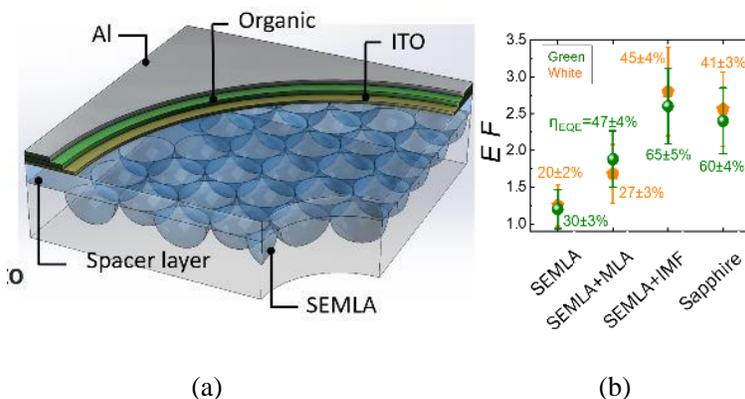
Figure 6-4. University of Michigan Sub-electrode Microlens Array Approach: (a) Device Architecture; (b) Light Extraction Enhancement Factor [46]
