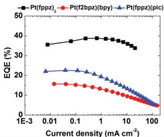
Figure 6-5. External Quantum Efficiency of Phosphorescent OLEDs with Pt-Based Emitters [51]
