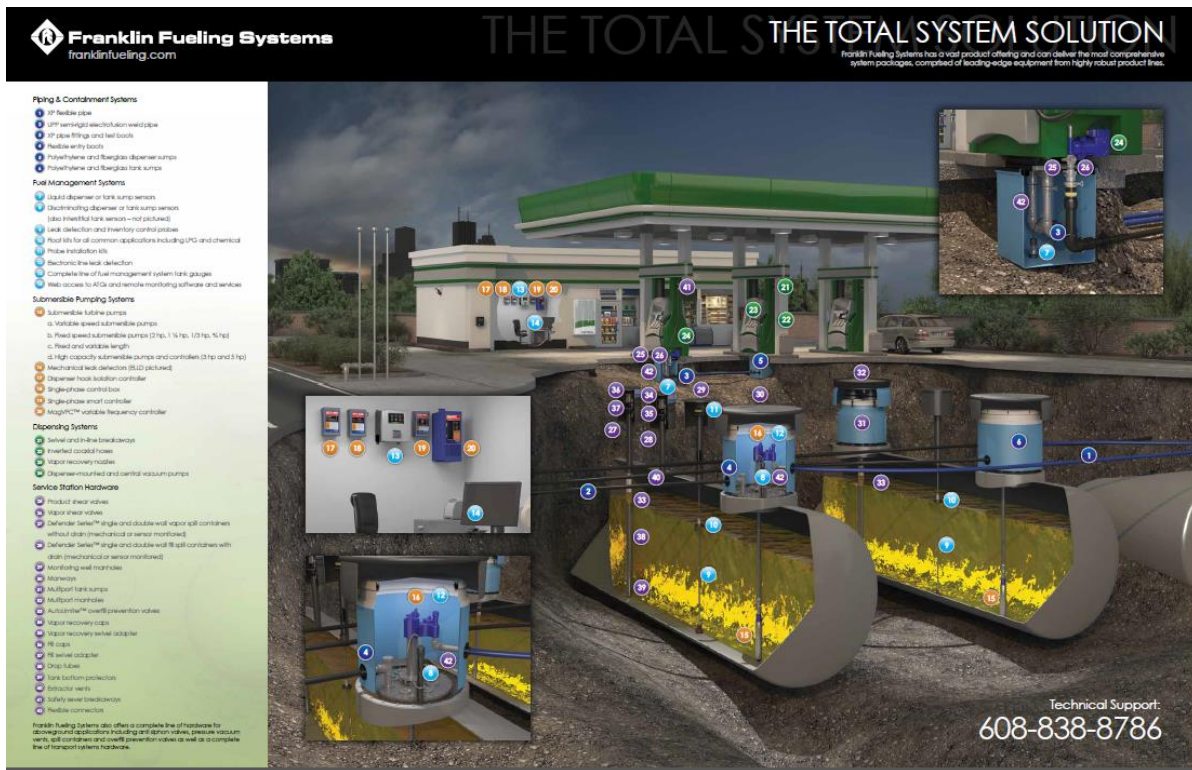
Figure 2-1. Overview of a retail refueling site. Image source: Franklin Fueling Systems.
