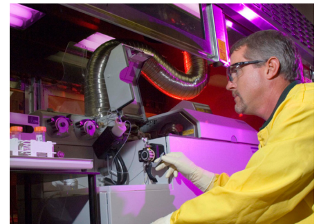
A lab employee performs technical oversight of an Inductively Coupled Plasma-Mass Spectrometer.
