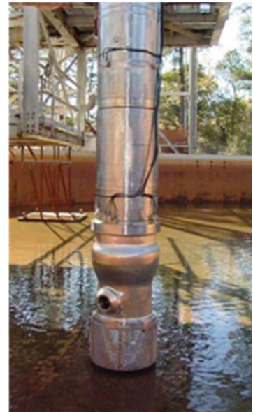
Figure 2.3-4: Submersible Mixing Pump in a Test Tank
