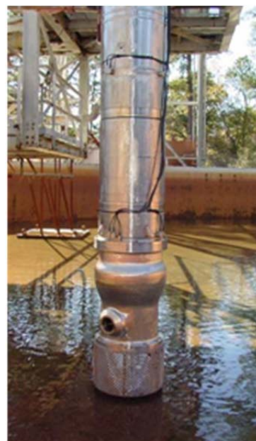
Figure 5.2-5: Submersible Mixing Pump in a Test Tank
