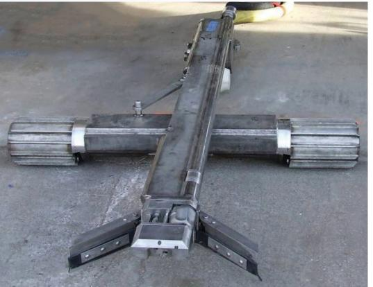
waste tanks. It sprays highly-pressurized water from a tiny opening made of specially selected material that can stand up to the water's pressure over time. The complete robot is 8 feet long and weighs approximately 800 pounds. The Sand Mantis' cross-shaped body can be collapsed into a straight line for insertion through the small openings in the top of a tank. Once inside, the robot unfolds and is remotely guided.
