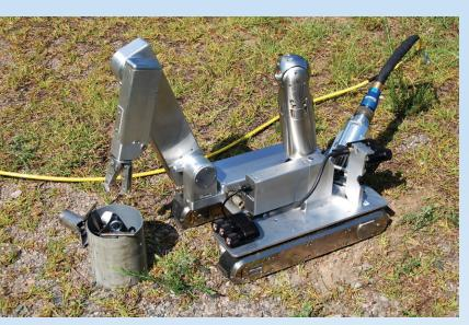
Frankie, a commercially available robot, was modified by SRR and moves across the tank floor on treads. Frankie's primary function is to scoop thin layers of residual material left behind from heel removal and cleaning processes. Frankie replaces a custom-built vial that was scraped along the tank floor; Frankie does a better job and with less risk to workers.
