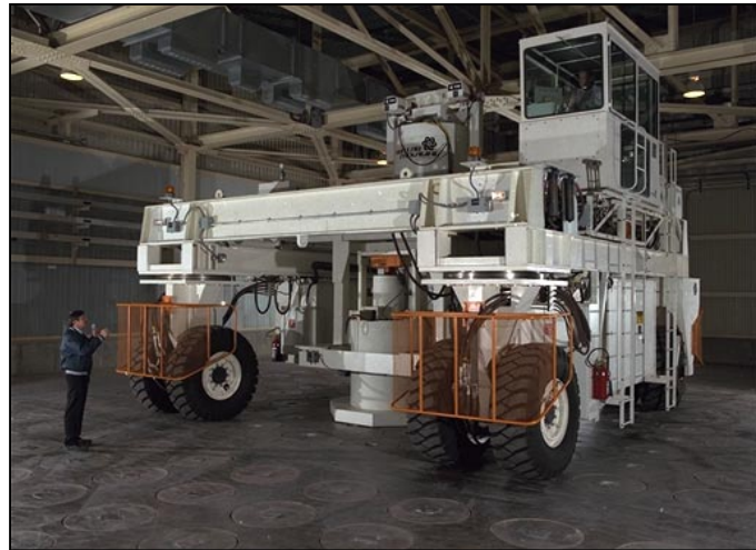
The Shielded Canister Transporter (SCT) moves highly radioactive canisters from DWPF to the GWSB. The SCT removes a round shield plug from the floor, lowers the canister into a vertical storage position, and replaces the shield plug.
