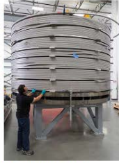
Central solenoid (CS) modules are in serial fabrication at General Atomics' Poway, CA facility.
