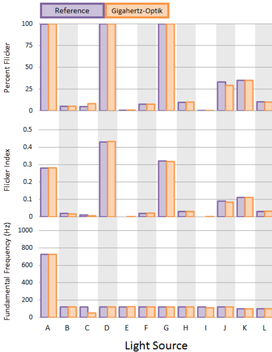
Figure 20. Gigahertz-Optik and reference meter flicker metrics for the various light sources tested.
