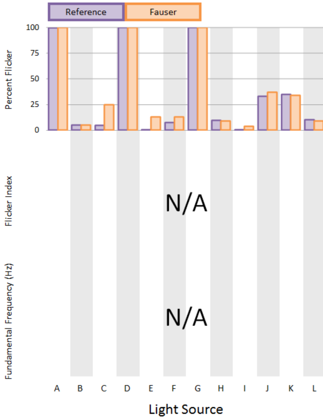
Figure 16. Fauser and reference meter flicker metrics for the various light sources tested.
