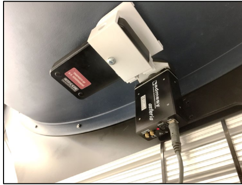
Figure 3. Handheld meter slid into place on flange, next to the reference meter.
