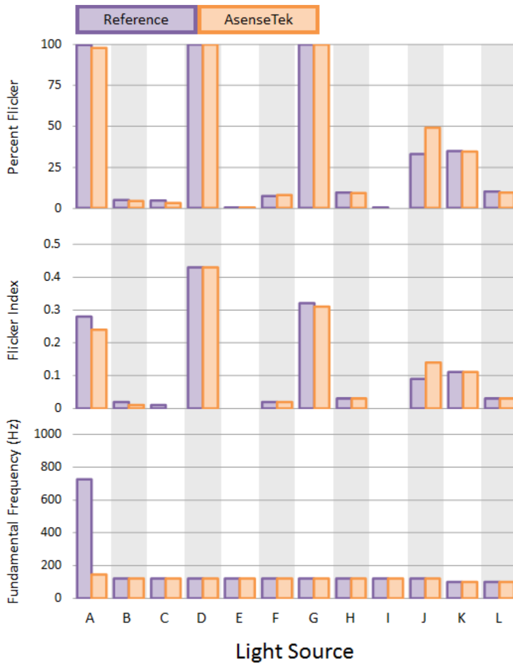
Figure 15. AsenseTek and reference meter flicker metrics for the various light sources tested.
