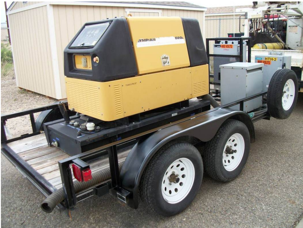
Figure 1. Olympian 20-Kilowatt Generator
