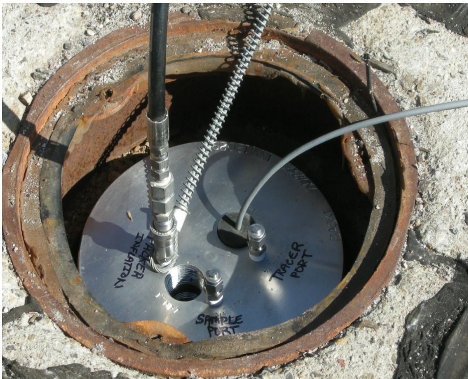
Figure 2.2-2 Permanent packer installed in borehole 54-24399 in August 2016
