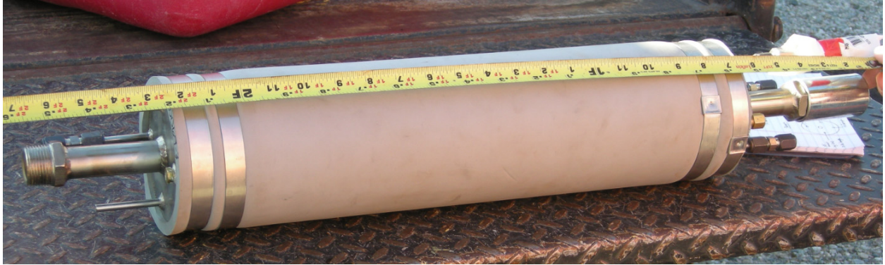
Figure 2.2-2 Permanent packer installed in borehole 54-24399 in August 2016
