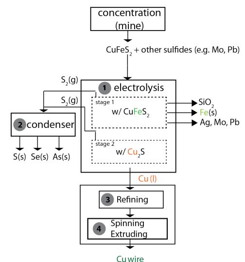
Molten sulfide electrolysis of copper concentrate involves a reactor that operates solely on electricity to produce liquid product amenable for a novel wire production process.
