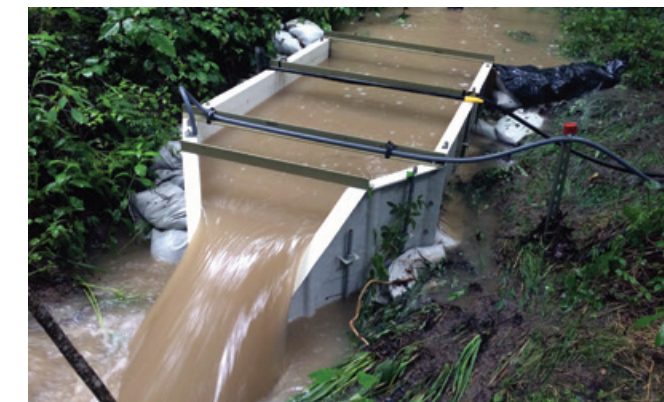
Flumes installed on the proposed EMDF site measure flow rates and general condition of the surface water
