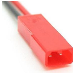
Figure 7. Team-provided connection to the manual shutdown interface
