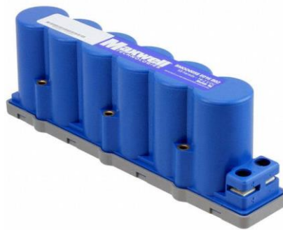
Figure 5. Competition-provided ultracapacitor storage element
