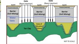
In Situ Treatment using Wall and Gate for Combined Hydrologic and Geochemical Control
