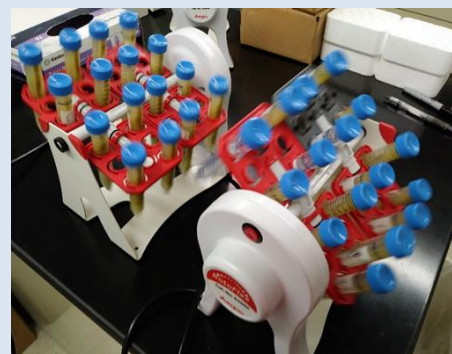
Tube rotator (L/S=10 mL/g, 1 g sample)
