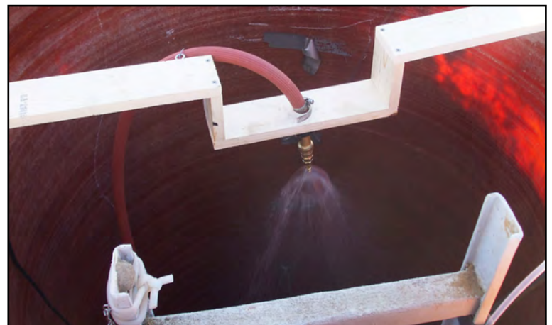
Figure 1. The first tests at the Mound system (left) used a small garden fountain pump attached to landscaping mist nozzles, with an air monitor to detect whether the contaminants were moving from the water to the air. The test was performed in a plastic box. The next test (right) used a larger pump and spray nozzle. Both showed that air stripping removed contaminants from the groundwater, and led to a larger air stripper at the Mound system (not shown).
