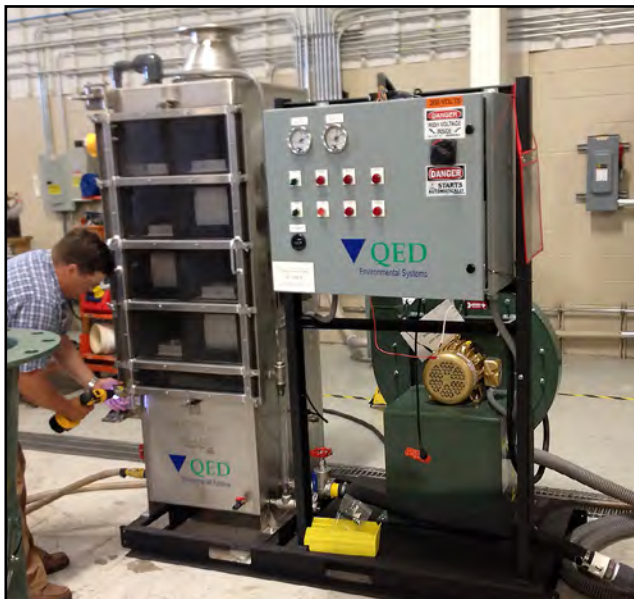
Figure 3. The new, commercial air stripper is shown in the left photo above, and will be housed in the shed shown in the photo on the right. The roof of the shed is angled to provide better solar-thermal exposure. The solar/battery conex from Figure 2 (see page 14) is visible in the background to the left of the shed.
