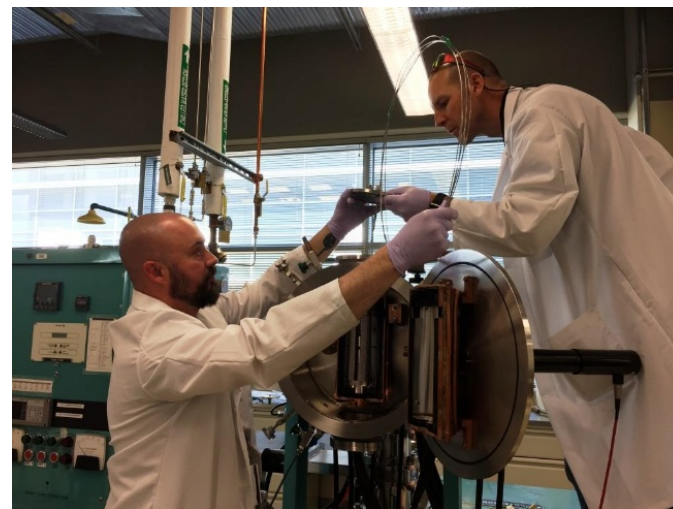
UT calibration in HTTL vacuum furnace
