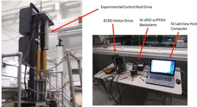
**Figure 4. ECRD motor drive, and National Instruments equipment used for implementing SPD-based closed-loop control.**
