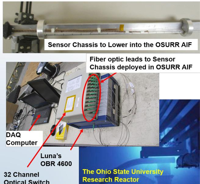
Figure 4. Test setup for irradiation tests at The Ohio State University Research Reactor (OSURR) (Top) Chassis holding 17 fiber sensors. (Middle) DAQ system with 32 channel switch. (Bottom) OSURR in operation.
