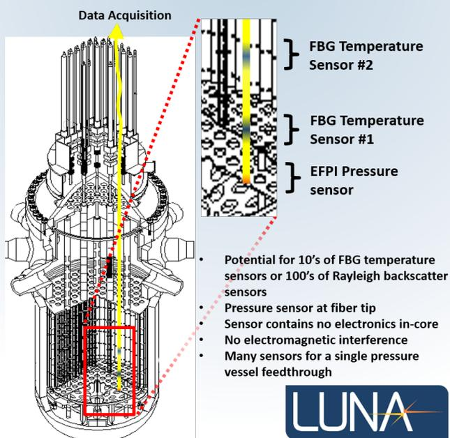
Figure 1. Concept diagram describing planned inline multipoint temperature and endpoint pressure fiber optic sensor.
