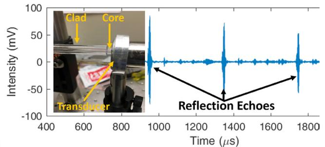
**Figure 3. Acoustic excitation and detection of “suspended core” acoustic fiber and reflection spectrum.**
