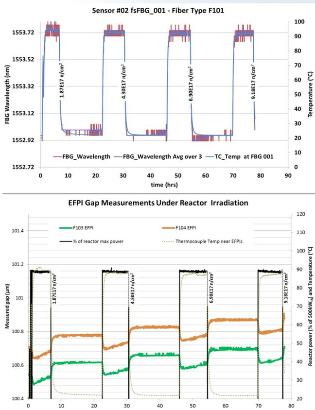
**Figure 5. Sensor measurements while being irradiated at OSURR. Irradiation occurred over four days with approximately eight hours of reactor operation each day. (Top) Comparison of FBG Wavelength and thermocouple response for F101 fiber type (Bottom) EFPI response during reactor operation.**
