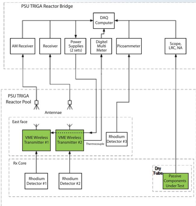
Figure 2. PSBR test configuration.
