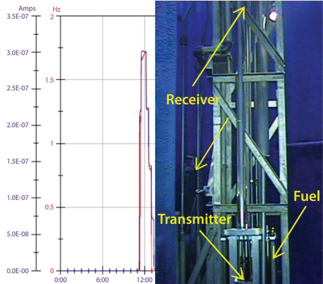
Figure 3. SPD output versus AM transmitter, and PSBR core.
