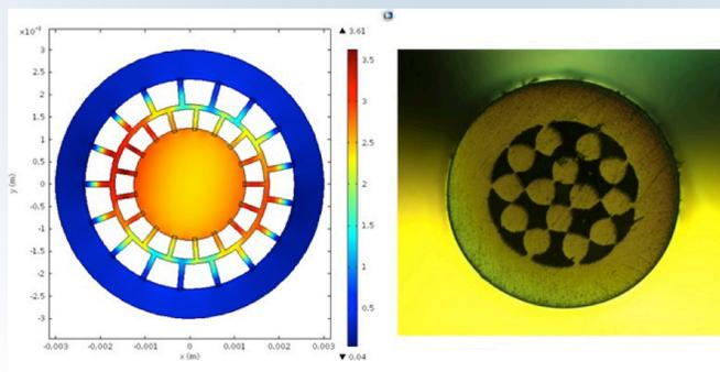
**Figure 2. (a) Theoretical waveguide modeling of fused silica acoustic fiber. (b) Optical micrograph of acoustic fiber fabricated on commercial optical fiber draw tower.**
