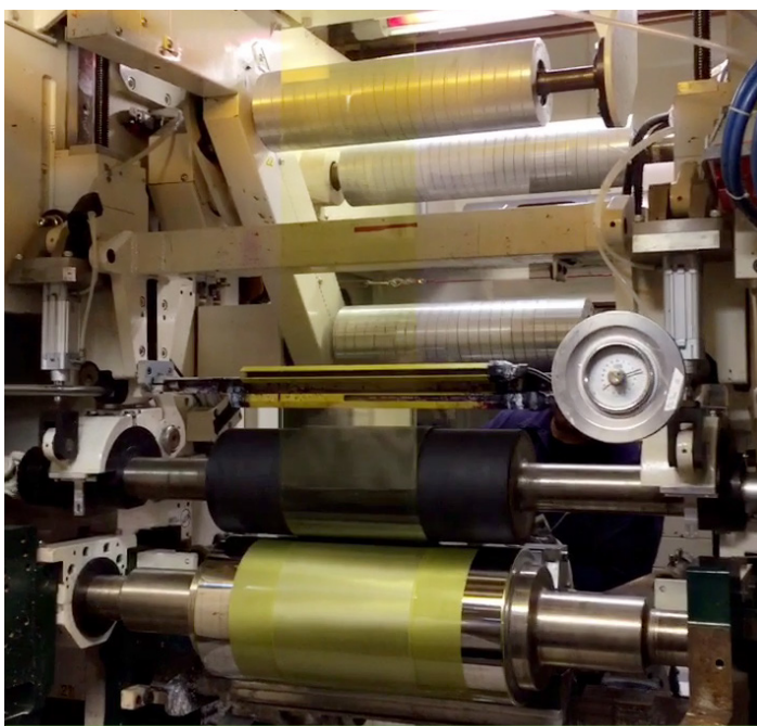
Roll-to-roll coating of perovskite ink at 100 ft/min on a polyethylene terephthalate substrate previously coated with indium tin oxide and a hole transport material.
