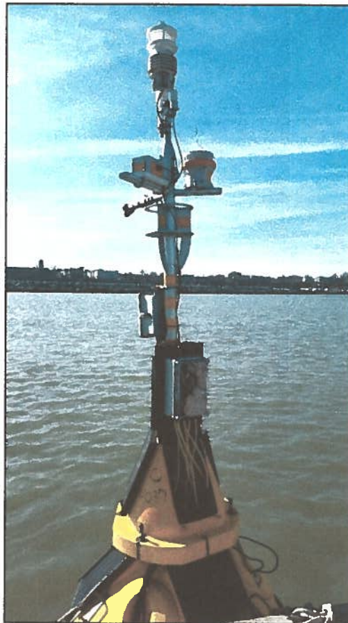
Figure 3. SM4 Bat Detector Deployed on a buoy for the Icebreaker Wind Project, showing microphones deployed at approximately 2m above the surface of the water
