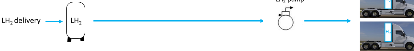
CcH 2 solution: direct fill of cryogenic fluid
