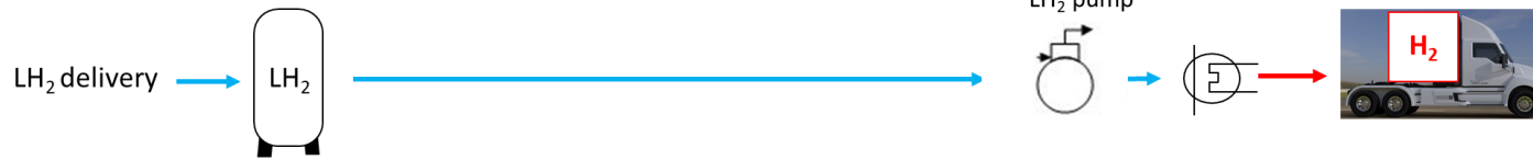
CcH 2 solution: direct fill of cryogenic fluid
