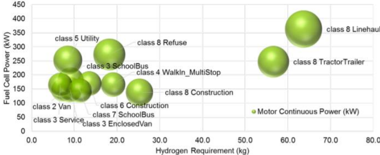
FIGURE 1. Fuel Cell and Hydrogen Tank Sizing Result for FCETS
