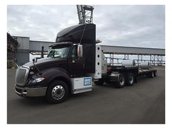
Range: 150 Miles Fuel Capacity: 20kg Horsepower: 442
