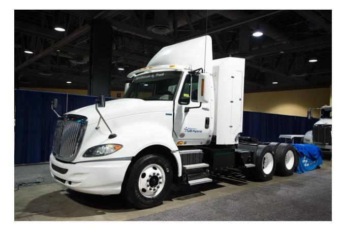
Range: 200 Miles Fuel Capacity: 25kg Horsepower: 429
