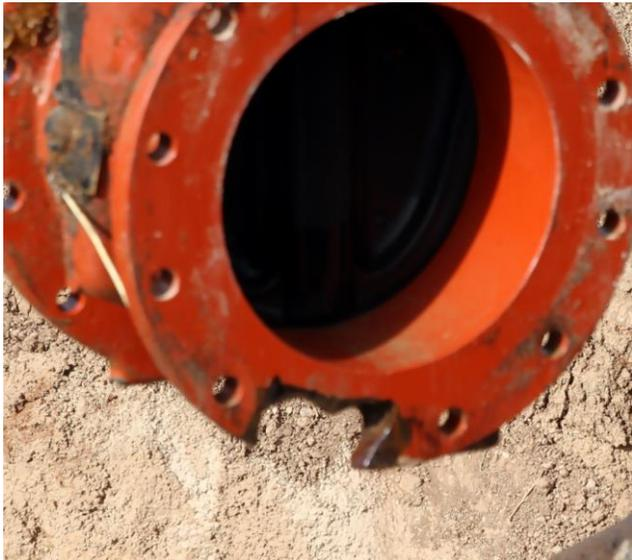
A section of the eroded valve flange
