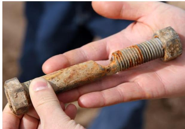
**Bolt cut from the water leak between the flange faces**
