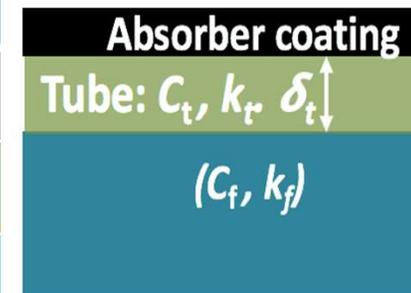
Thermal penetration depth:  $L_p = \sqrt{2 \alpha / \omega}$
