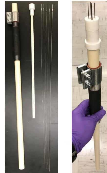
Pilot-scale multi-electrode array sensor for molten salt monitoring
