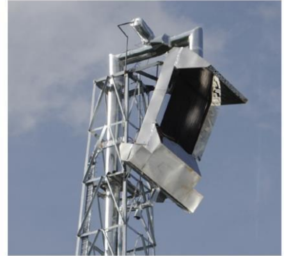
Fig. 5. 1.2 MW th tubular sodium receiver at Vast Solar's Jemalong Solar Thermal Station.
