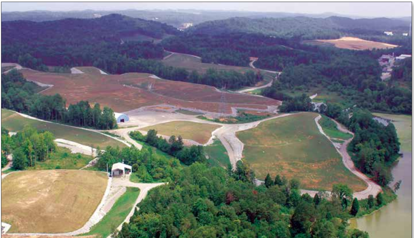
Melton Valley is a large area near ORNL that was a waste repository for many years. Remediation was completed in 2006 but long-term stewardship is required due to the long-lived radionuclides that will be a human health and environmental concern for thousands of years.
