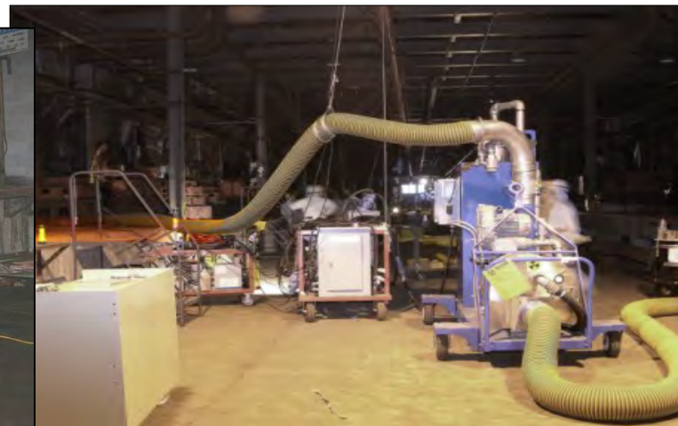
Uranium hexafluoride vent, purge, and drain operations
