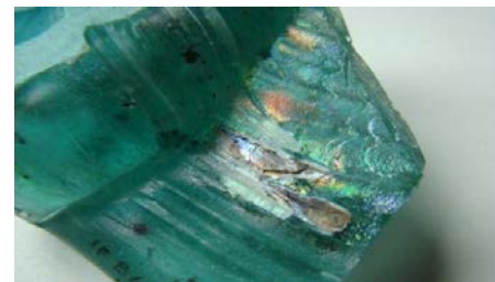
Ancient glass from the Roman ship-wreck ~1800 y ago, giving understanding of glass corrosion over long time scales
