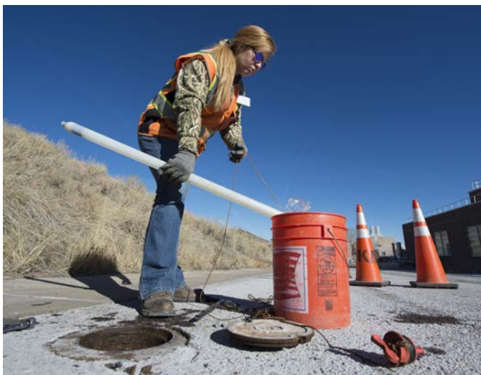
A subcontractor measures water levels and takes groundwater samples north of the Field Testing Laboratory Building.
