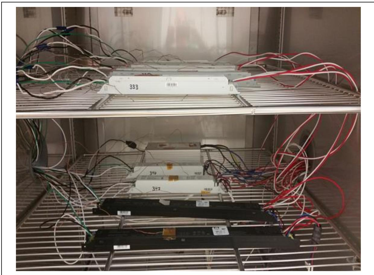
Figure 3-1. Configuration of the DUTs during AST exposure and the connecting wires to the ac source and the LED loads.
