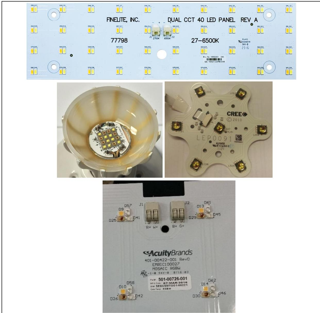
**Figure 1-6.** Examples of LED modules comprising multiple LED assemblies for use in TWL devices.
