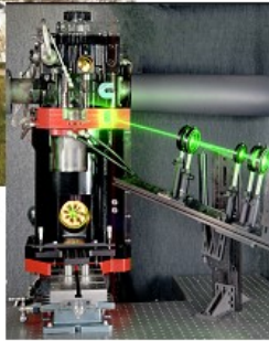
SNL optical engine with laser and optical diagnostics
