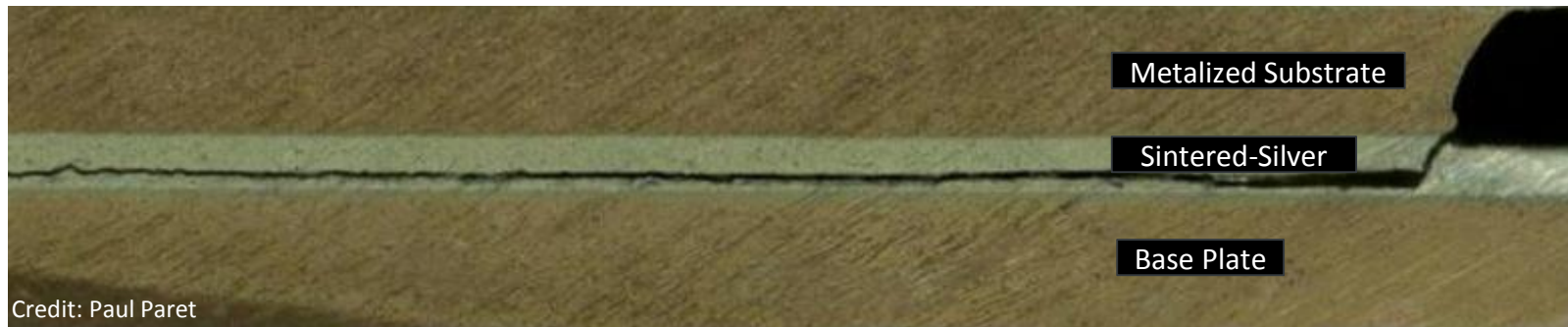
Crack Propagation in Pressure-Assisted Sintered Silver
