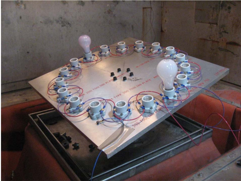
Figure 2.1. Stress Test Board, Showing Electrical Wiring
