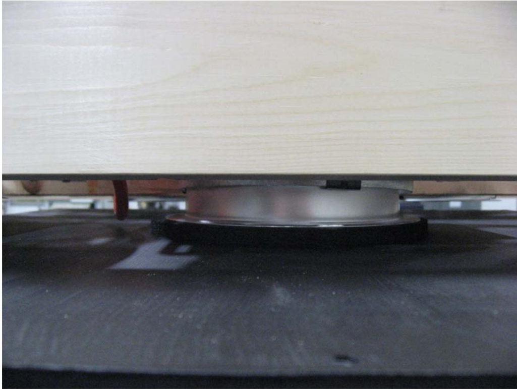
Figure 2.7. Foam Seal Mated to Downlight on Top of Measurement Chamber
