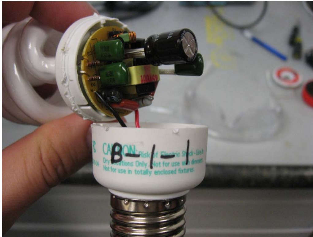
Figure 4.1. CFL Disassembly for Failure Analysis
