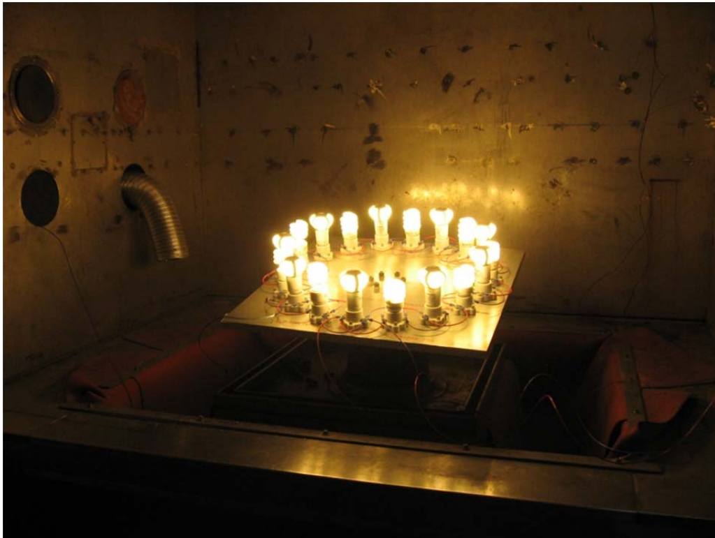
Figure 3.1. Energized Test Board Prior to Stress Exposure
