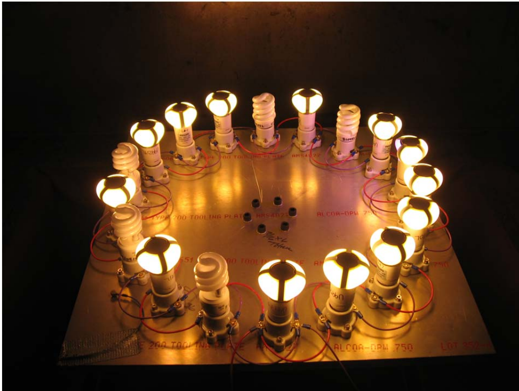
Figure 3.2. Energized Test Board Following Completion of All Test Steps
