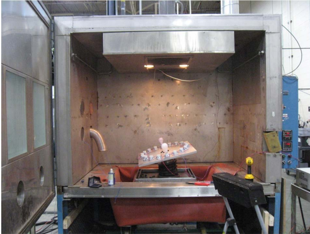
Figure 2.3. Environmental Chamber With Mounted Stress Test Board
