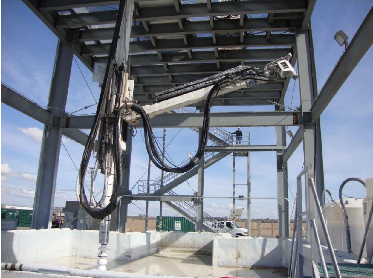
Figure 2-22. Sluice-Mode Mobile Arm Retrieval System In-Tank Components.
