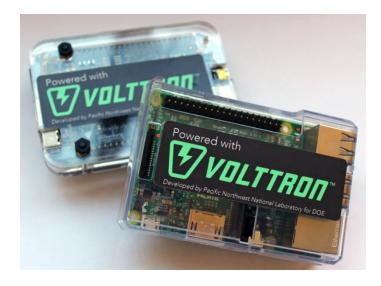
The economic dispatch and supervisory control software will be deployed on the versatile and secure VOLTTRON™ distributed control platform, hosted on a low-cost (<\$200) hardware and integrated with the existing building automation system
