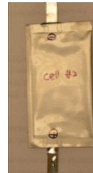
Flexible solid-state supercapacitor
