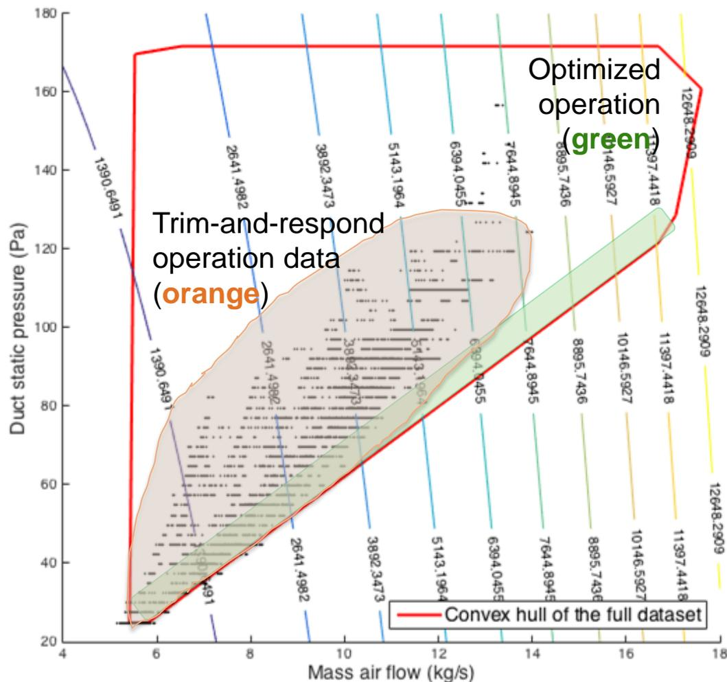
Learning algorithm emphasizes accurate representation of the fan power consumption model at boundary corresponding to optimized operation
