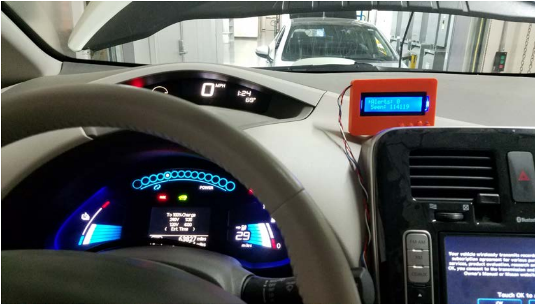
Figure IV.4.3 - DSM Installed in Nissan Leaf – Showing Status
