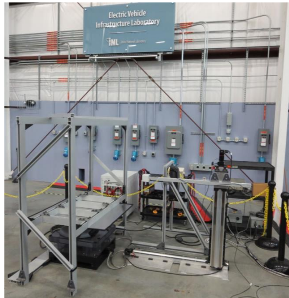
Figure V.2.1 - Bench Testing of Wireless Charging Interoperability to Support SAE J2954 (Source: INL)
