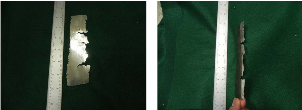
Figure I.10.1 - Fe-6.5Si-xB steel thermomechanically processed and rolled at room temperature to a reduction of roughly 77% reduction in thickness.
