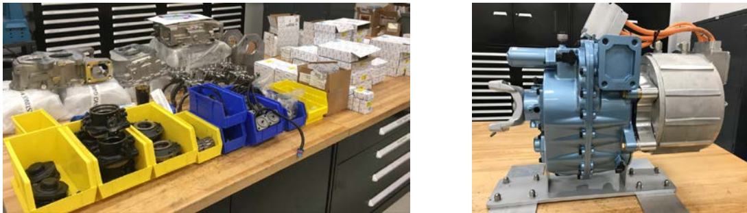
Figure III.4.1 - Left: Components of 4-Speed AMT are laid out before the assembly. Right: Eaton 4-Speed EV-AMT display unit integrated with a UQM Electric Motor.
