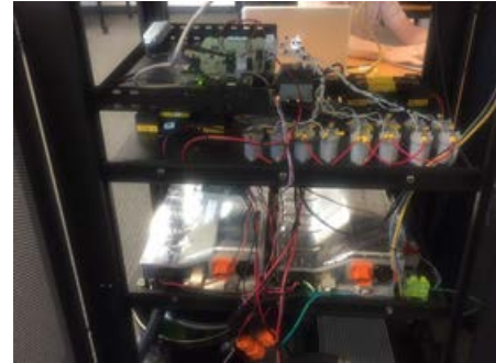
Figure III.1.4 - SPIN Rack Mounted Unit for Power Controls and Analytics Algorithmic S/W Integration and Testing
