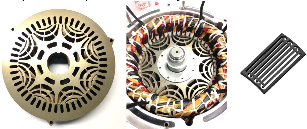
Figure I.3.4 - ORNL synchronous reluctance motor prototype stator/rotor (left), stator/rotor assembled and installed in housing (middle), and cooling insert (right).
