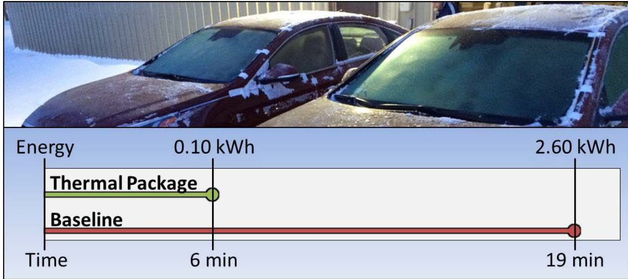
Figure V.4.2 - Results of stationary defrost cold-weather field evaluation for both the baseline and thermal load reduction system
