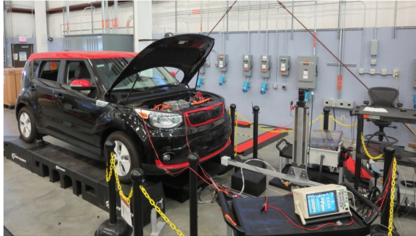
Figure V.3.1 - Testing and Evaluation of the Hyundai / Mojo Mobility WPT system on a Kia Soul EV at INL’s EVI lab (Source: INL)
