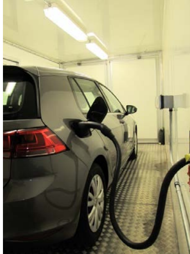
Figure III.6.2 - A 2015 Volkswagen e-Golf DC fast charging in the temperature chamber at Intertek in Phoenix, Arizona/Intertek
