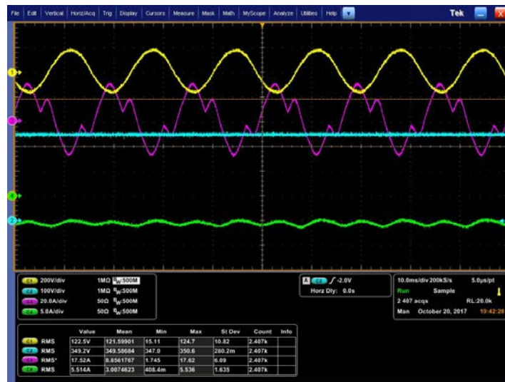
Figure II.1.6 - 120Vac charge waveform, Vdc=350V (CH1: Vac, CH2:Vdc, CH3:Iac, CH4:Idc). Load is 400W incandescent light bulbs + 1400W microwave oven
