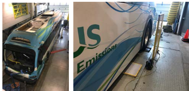
Figure III.4.5 - Vehicle mounted on NREL’s heavy-duty chassis dyno with all data acquisition implemented and ready for testing
