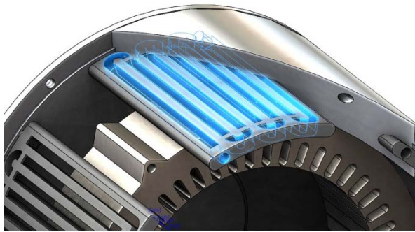
Figure I.15.6 - Cross section view of ORNL stator cooling jacket for computational fluid dynamics thermal and fluid analysis at NREL (left), transverse rupture test results comparing new and prior generation Ames magnets (right).
