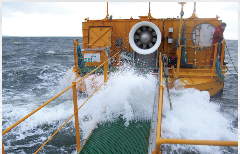
The OE Buoy is designed around the oscillating water column principle. Its turbine captures the energy of the wave and the generator converts this energy to electrical power. A full-scale commercial prototype will have a capacity rating of 1.75 MW.
