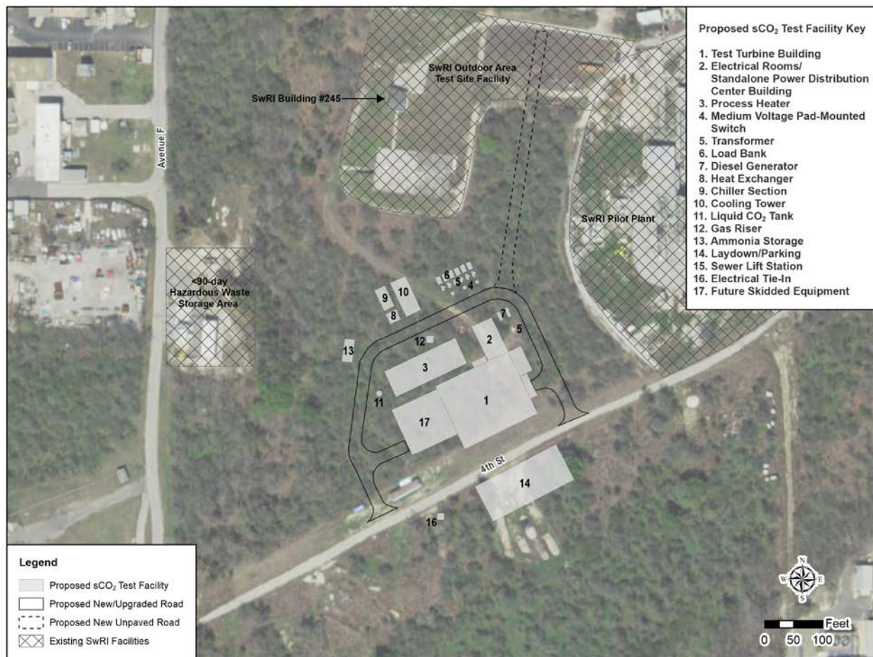
Figure 2-3. Proposed sCO 2 Test Facility General Arrangement Plan
