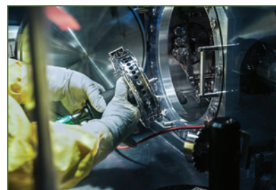
SRNL's TRITON™ thermal ionization mass spectrometer sample wheel.
