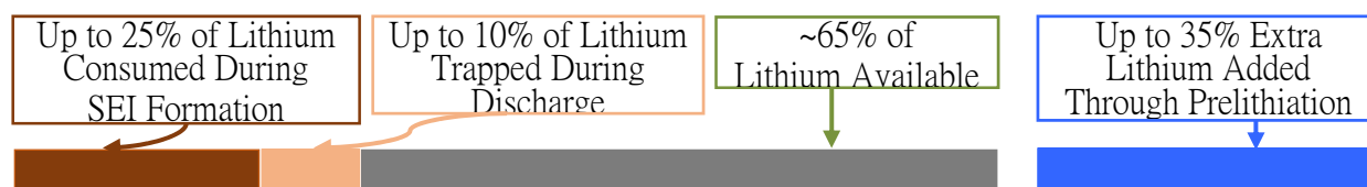
Figure IV-347: Silicon anodes consume and trap significant amounts of lithium, reducing first cycle efficiency and cell-level energy. Current lab-scale prelithiation methods add extra lithium and address first cycle loss – but are not scalable
