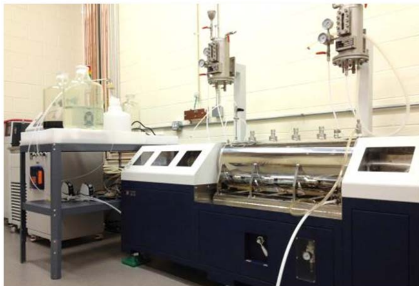
Figure IV-262: Installed 10 L Taylor Vortex Reactor
