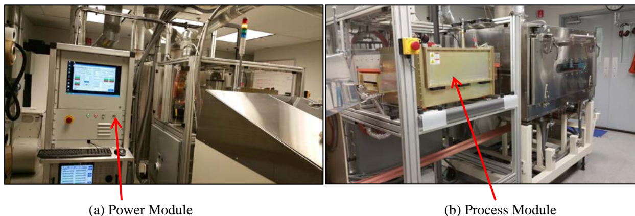
Figure IV-352: Digital image of the ADP Pilot oven installed at Navitas. The Power Module (a) delivers VFM power through the waveguide connected to Process Module (b), which is placed between the coater and the standard convection oven
