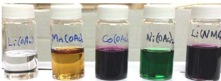
Figure IV-332: DESs of different metal acetate hydrates and that of a mixture to make LNMC materials
