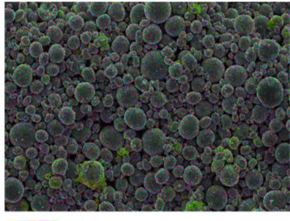
Figure IV-155: SEM and EDS mapping images of LaPO<sub>4</sub> coated NMC 622 with 5% coating solution amount to the sample mass
