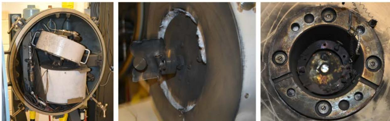
Figure IV-91: ARC conditions from attempted evaluation of 18650 cells using NCM523 vs. 10 and 15 wt% nanosilicon
