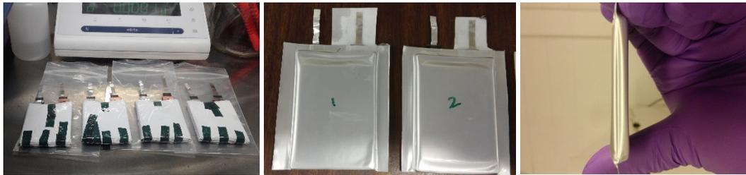
Figure IV-239: Photos of the final delivered full cell
