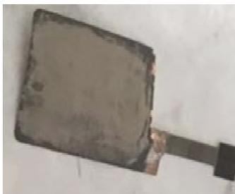
Figure IV-236: SLMP coating on 12 cm<sup>2</sup> pouch cell with the optimized disperse agent, i.e.m 0.5 wt% SBR and 0.5 wt% PST in xylene solution
