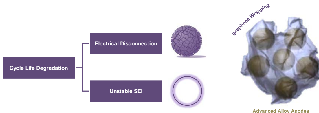
Figure II-34: Si-anode failure mechanisms (left), SiNode graphene-wrapped advanced silicon anode architecture (right)
