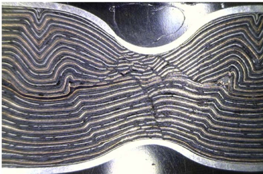
Figure III-46: Internal shear faults and folding of electrodes in a prismatic cell under pinch test [4]
