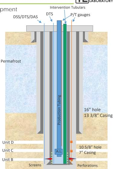
Located between two monitoring wells: design in development
