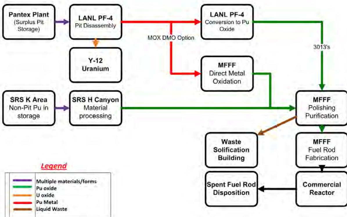
**Figure 3. Basic Flow Diagram for the MOX Approach**
