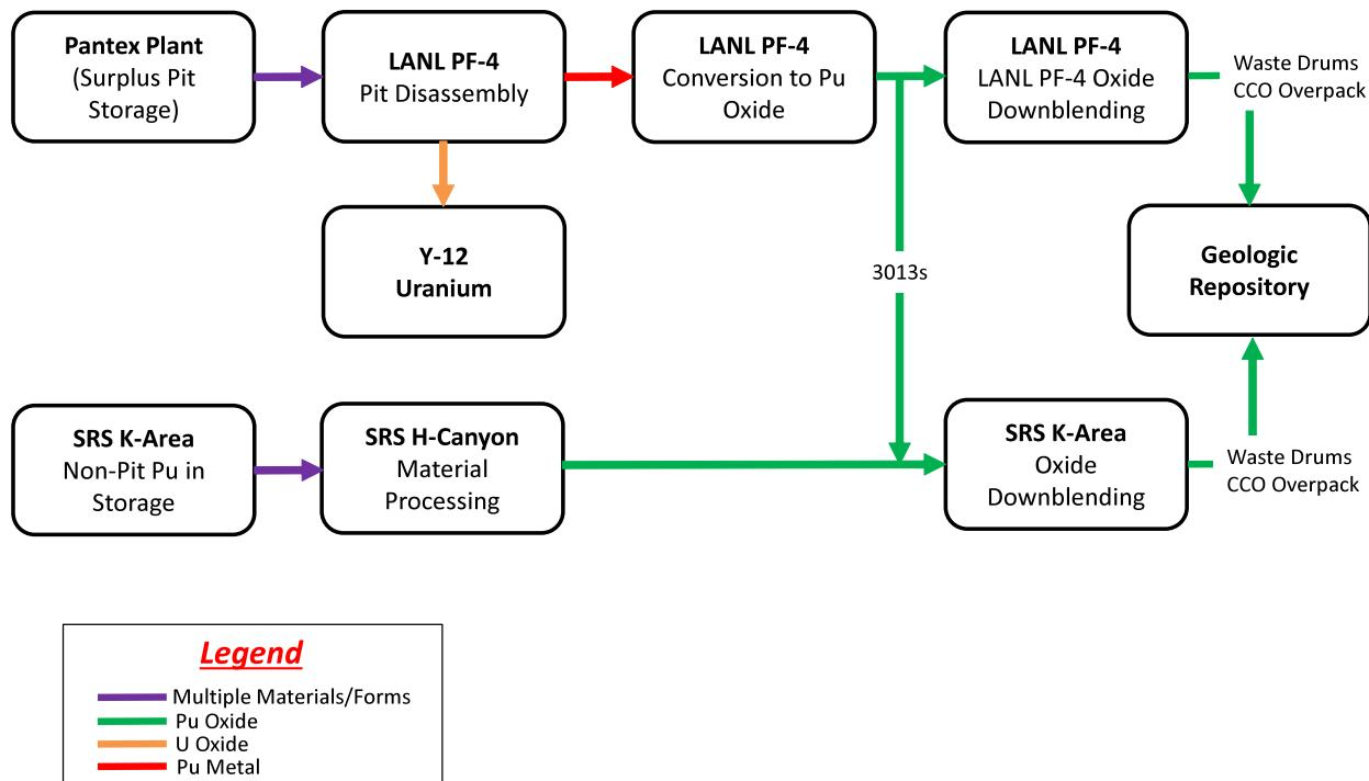
**Figure 5. Basic Flow Diagram for the Dilute and Dispose Approach:** This figure shows the major material flows for the base Dilute and Dispose approach as well as one variant, described later. Under this variant, LANL also dilutes material as a second production site, working in parallel with SRS.
