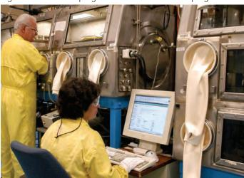
perform plutonium metal preparation and recovery operations. Foundry, machining, welding, and assembly operations also are required for pit manufacturing, as well as a complete suite of nondestructive analyses to ensure product acceptability.
